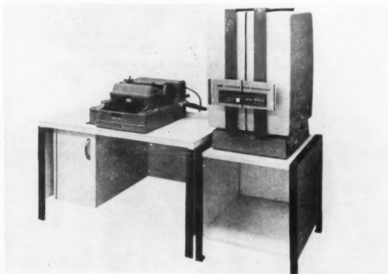
PB 250 by Packard Bell is one of the smallest high speed digital computers available. In this desk-side model both data and commands required for computation are stored in a homogeneous memory. Maximum operation rate is over 40,000 instructions per second, and a 22 bit square root problem can be completed in only 252 microseconds. Cost $30,000; monthly rental $1,000.
